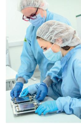
Researchers assembling particle detectors inside the 120m<sup>2</sup> clean room at the IIHE.
